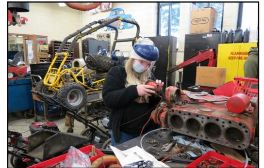
working on snow blowers and small engines of all kinds. The second year is rebuilding a small block Chevy with new pistons, rings, cam, bearings,
